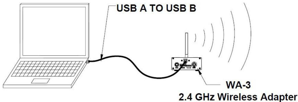
Connect the WA-3 to the USB on the laptop computer with a USB-A to USB-B cable (R-015-606). Laptop will assign a COM port number that must be selected within SynchroMM as the input. (Refer to instructions in the back of this manual on locating the assigned COM port.)
