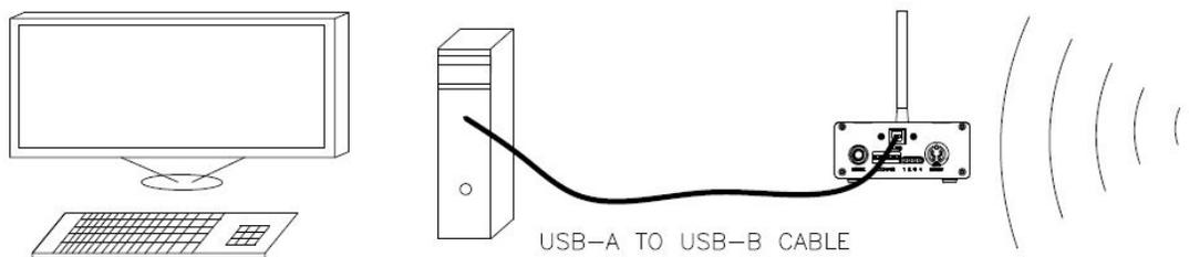
Connect the WA-3 to USB on the Display Link Plus (DL+) computer with a USB-A to USB-B cable (R-015-606). Power comes to the WA-3 via USB from the computer. Computer will assign a COM Port number that must be selected within Display Link Plus (DL+) as the input. (Refer to instructions in the back of this manual on locating assigned COM port.)
