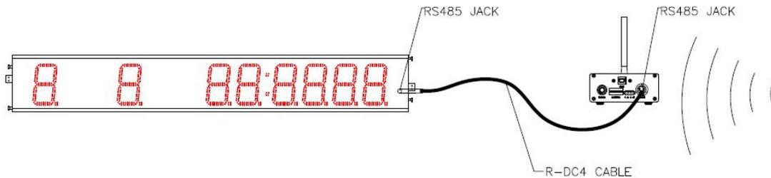
To display data on the LED-R scoreboard(s) or P01-style mini scoreboard(s), connect the WA-3 to a scoreboard with an R-DC4 cable. Power comes to the WA-3 from the scoreboard. If you have multiple scoreboards, connect them to each other with R-DC4 cables (ordered separately).
