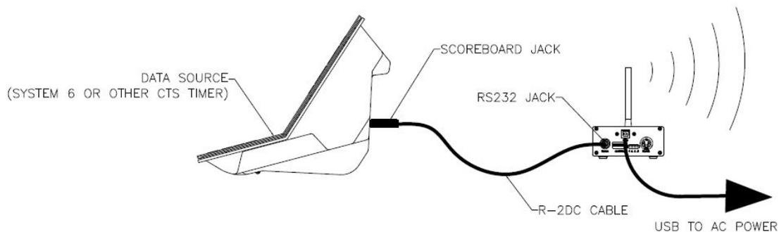
Connect the WA-3 to AC power with the USB power adapter, and to the System 6 with an R-DC cable.
